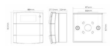
The FC420CP-I may be fitted to a standard (surface mounting) call point back box which is available separately.
