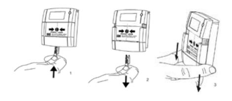
A test key is provided with each MCP to allow easy testing of the switch mechanism and wiring, without breaking the frangible element. The key is inserted into a slot in the base of the MCP, allowing the frangible element to drop away from the switch, thus activating it and registering an alarm at the CIE. Note: the key should not be left with the MCP after commissioning, but may be left inside the CIE for convenience.
