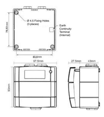
Ensure the cable entry holes are in the vertical plane, with either the single or double entry holes at the top.
